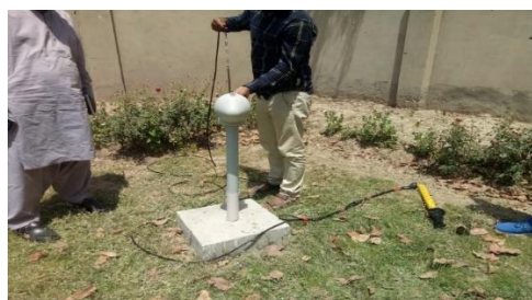
Figure-6: CTD sensor installed at Jalwala head (ESC Tail)
